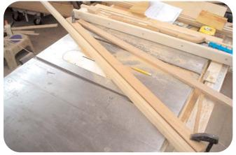
The table saw must be set up accurately to get the correct depth and width of the hollow. To assist in getting things right, cut a length of scrap lumber to the same width
