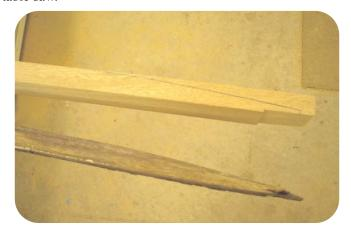
Now look at the backside of the original quarter rail and you will see it is slightly hollowed out leaving an eighth-inch wide edge on either side. This is so the quarter rail fits snugly to the slightly curved hull. Unless you have a shaper and a bit specific to the size for the hollowed area, an alternate tool must be used, and that would be a table saw. To do this, the stock must be run through the table saw at an angle as shown in the picture below.
