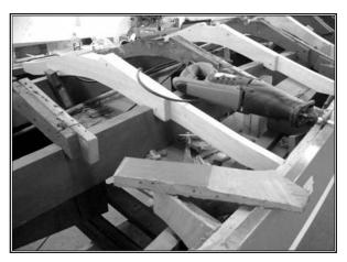
Additional tools required to clear out all of the 3M5200 and remaining frame wood and will be a heat gun to soften 3M5200, a chisel and mallet, planes, and whatever tools you can find to get the frames clear of debris.
