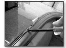
not to slip off of the staple. If you slip off the staple, you are likely to drive the staple lifter into the varnish and make an ugly gouge in the deck. Learn from my mishaps. Often, only one side of the staple will come up. If so, use a pliers to pull it out the rest of the way. When you get the hundreds of staples out of the hideum, there will still be the crash pad upholstery with as many, or more, staples to remove.
