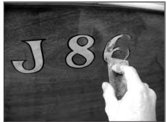
scraped off, avoid passing over that spot again. When you think you have all of the lettering scraped off, wipe the area down with alcohol and inspect it closely with good lighting for little specks and spots that have been missed. They will be there and will show up really well under new varnish if they are not removed.
