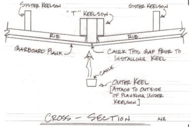
The sheets of plywood on the boat's bottom either side of the centerline are called the garboard planks. They come together at the centerline and are nailed and screwed into the keelson and ribs. Often times, there is a small gap where the two garboards join side to side. At the factory, a flexible marine caulk was run into this gap. This, in turn, was covered by the outer keel and stem. None of the wood was pre-primed or sealed prior to assembly.
