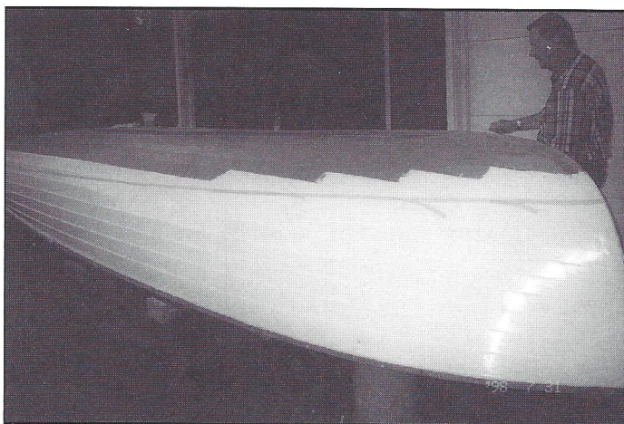
Hull exterior work nearly finished with application of anti-fouling paint.
