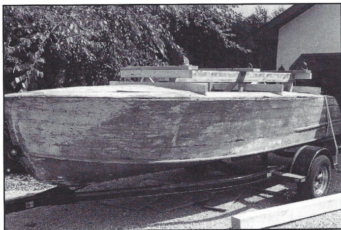
Jerry's 1950 Century SeaMaid is prepared for rolling over with the cradle screwed to the hull
