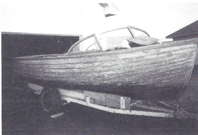
Sides stripped of paint
