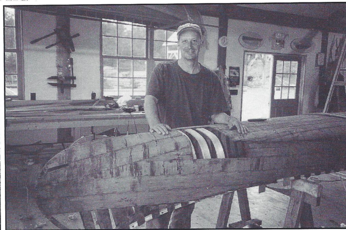
Dave Osborn showing his canoe with three new ribs and several planks removed.
