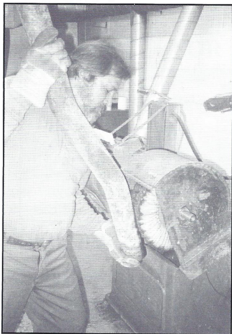
Bill McClure, Buffer, Polisher working on an exhaust pipe from a Chris Craft
