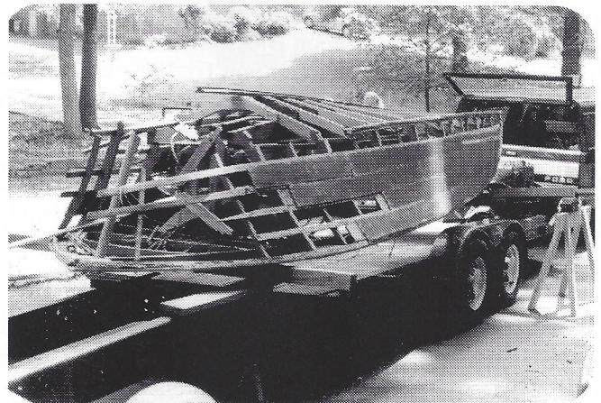
Century #6, May 2000, South Carolina 1956 Arabian - very derelict. Not original bottom frames. Missing lots of original planking.
