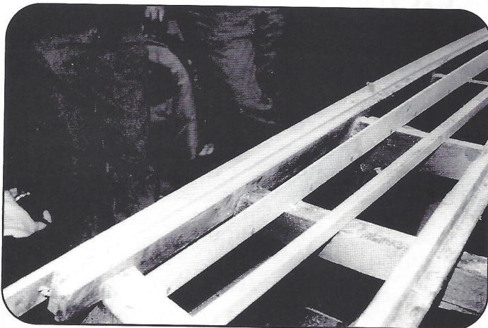
View showing the laminated chine and parallel mounted router guide.
