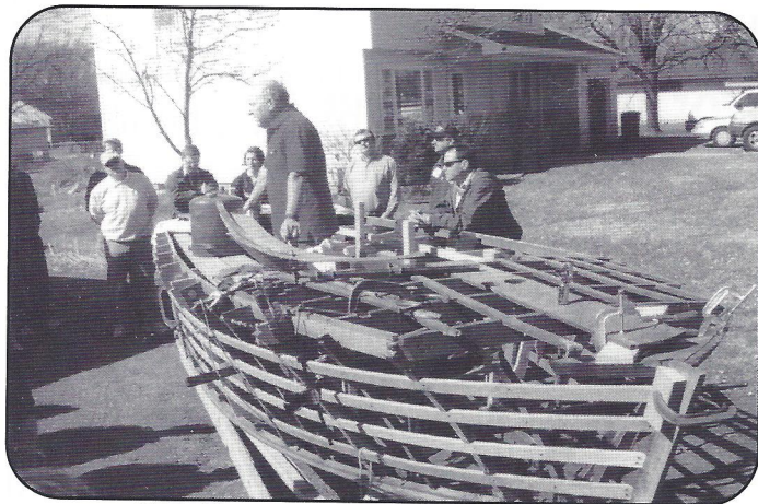
Bob Buttery explains the set up for putting in a gunnel clamp.
