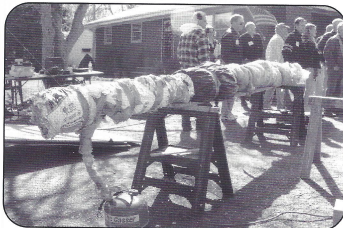
Bob's homemade steam box that is heating the clamp.
