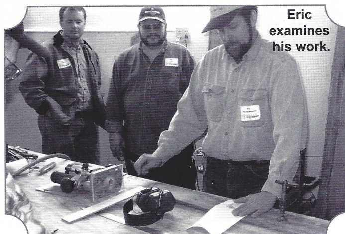
Eric demonstrates using a router to shape a joint
