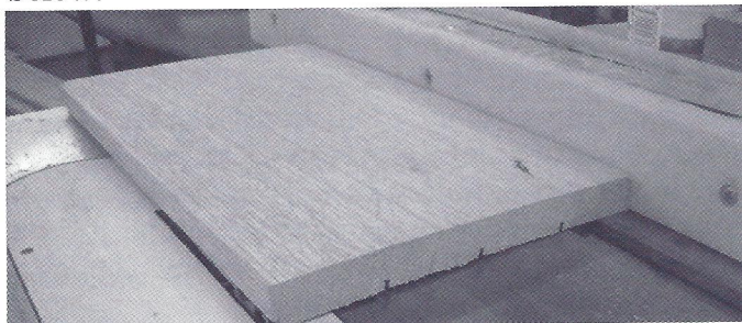
Cut seams 1/3 the thickness of the plank.
