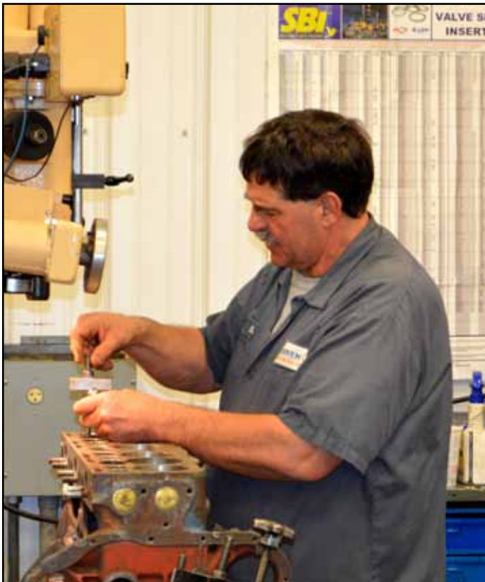
Keith walks us through the process of placing hardened valve seats in an older marine engine.
